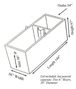
(Septic Tank drawings not to scale. Tank height is figured from bottom of tank to top of lid. Inlet and Outlet is figured from bottom of tank to bottom of inlet or outlet)
